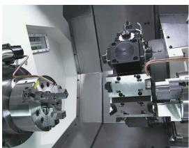
The space within the machining zone has been maximized to prevent any tool interference and provide the utmost flexibility and substantially reduce any chance of collision between the cutting tools and the machine.
